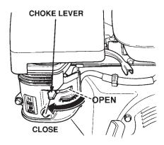
Figure 11. Choke Lever
